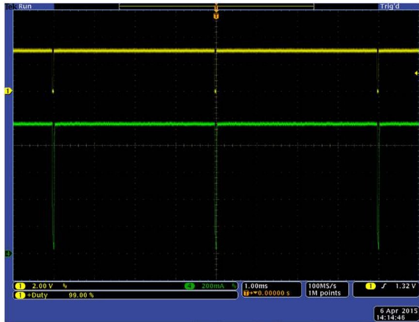
Figure 8. 99% Duty Cycle 250 Hz PWM Dimming, Top = PDIM, Bottom = LED Current
