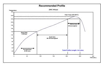
The recommended reflow profile for R276 made with SAC alloys is shown here. This profile is simply a guideline. Since R276 is a highly active solder paste, it can solder effectively over a wide range of profiles. Your optimal profile may be different from the one shown based on your oven, board and mix of defects. Please contact Kester if you need additional profiling advice.
