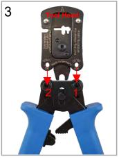
Open the handles and insert the tool head into the open holes.
