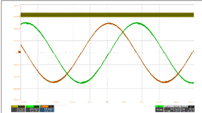
Figure 8-11. 1/256 Microstepping With smart tune Ripple Control Decay
