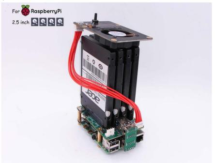
The Dual SATA HAT utilizes two high-performance JMS561 (one JMS561 for the Dual SATA HAT) and provides up to 400MB/s read/write performance with four disks in RAID0 mode.
