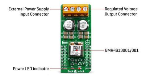
It is possible to monitor a wide variety of parameters through the PMBus interface. Fault conditions can be monitored using the SALERT pin, which will be asserted when any number of pre-configured fault or warning conditions occur. It is also possible to continuously monitor one or more of the power conversion parameters including but not limited to the following:
