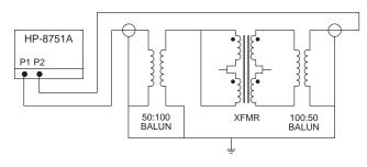
5. Crosstalk Attenuation — In the dual packages, which contain transmit and receive transformers side by side, sufficient crosstalk attenuation is achieved by the inherent characteristics of the toroid cores as well as by their proper positioning. The crosstalk attenuation is typically 50 dB or better from 100 kHz to 10 MHz. This result was established with the test circuit shown below.
