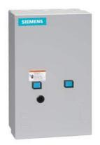
2-speed 3-phase motor starter Size 0 Two separate windings Constant or variable torque Solid-state overload relays Low SPD OLR range 3-12A High SPD OLR range 3-12A 110V 50HZ / 120V 60HZ coil Enclosure NEMA type 1 Indoor general purpose use
