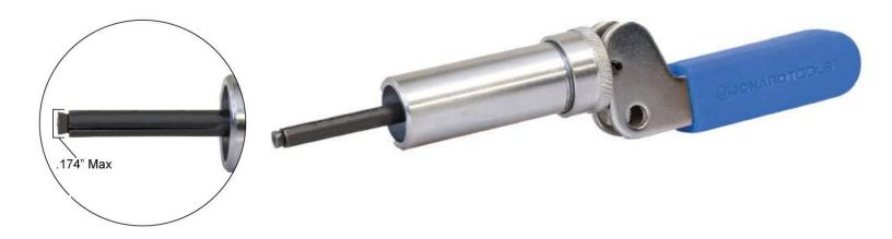
The Jonard Tools TTB-6 Barrel Lock Plunger Key is designed to unlock Channell LK03029817 and Highfield 93180775-S CATV barrel locks quickly and easily. It only works with these 2 types of locks with inside diameters from 0.176" to 0.196" (do not try to use for other purposes as it will not work). This barrel lock plunger features the following:
