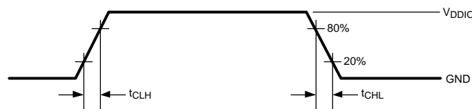
Figure 3. LVCMOS Transition Times
