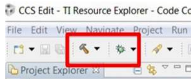
Figure 25. Build Project Files Buttons
