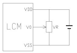
V<sub>DD-</sub>V<sub>0</sub>: LCD Driving voltage VR: 10k~20k
