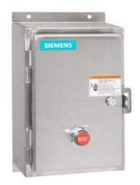
Non-reversing motor starter Size 3 Three phase full voltage Solid-state overload relay OLRelay amp range 25-100A 110VAC 50HZ / 120VAC 60HZ coil Combination type Water/dust tight non-corrosive
