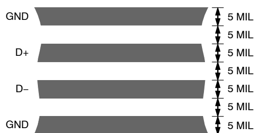
Figure 23. Typical Arrangement of Signal Tracks
