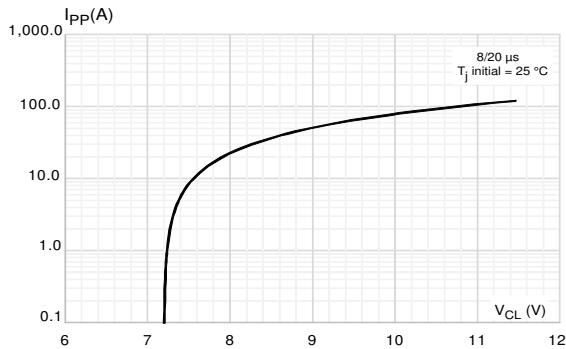
Figure 5: Peak pulse current versus clamping voltage (maximum value)
