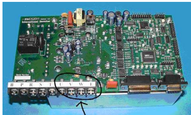
Figure 4. Motor Wiring Connection
