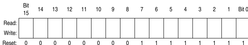
Figure 4-4. Stack Pointer (SP)
