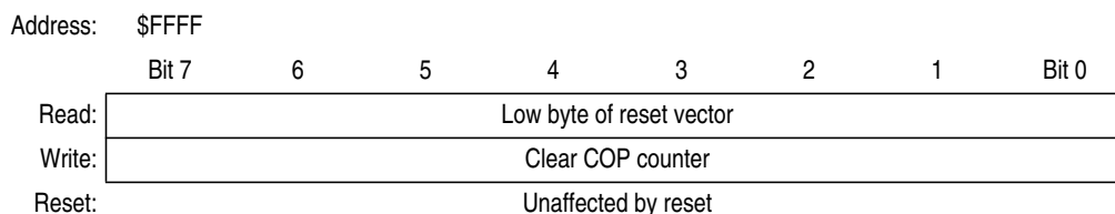
Figure 19-3. COP Control Register (COPCTL)
