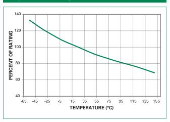
1. Re-rating depicted in this curve is in addition to the standard re-rating of 20% for continuous operation.
