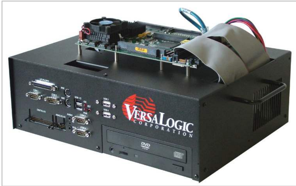
Figure 10. Example EBX Board Installation
