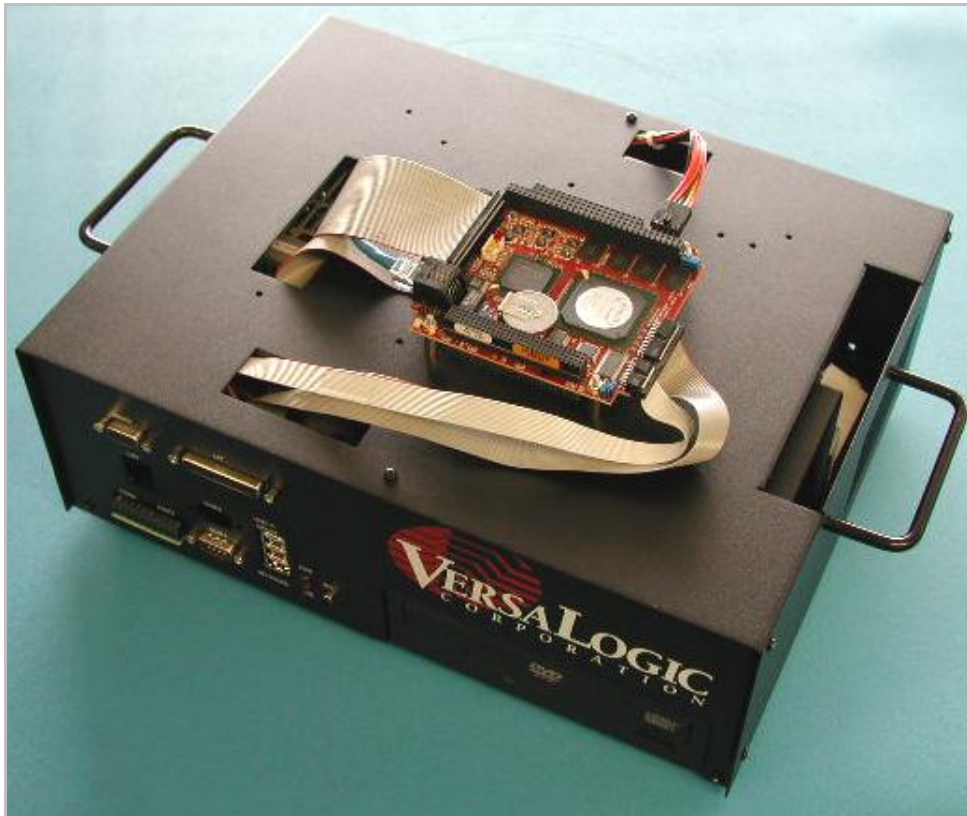
Figure 9. Example PC/104 Board Installation
