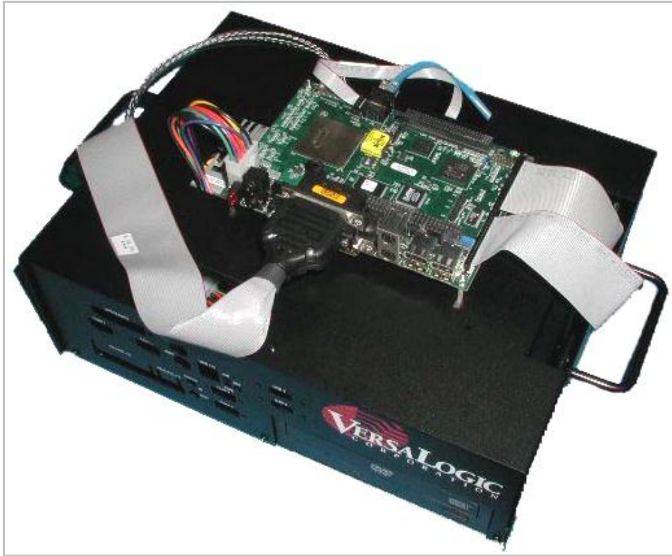
Figure 11. Example EPIC Board Installation
