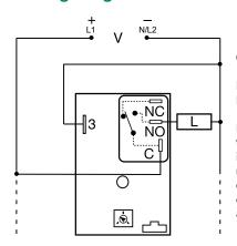
C = Common, Transfer Contact NO = Normally Open L = Load
