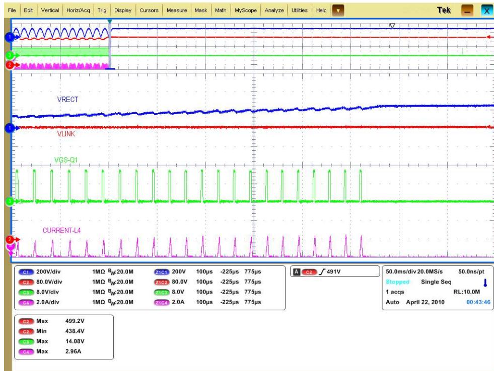
Figure 29. Transient — 115W to Zero Load at 10W/μs, Vin = 277VAC
