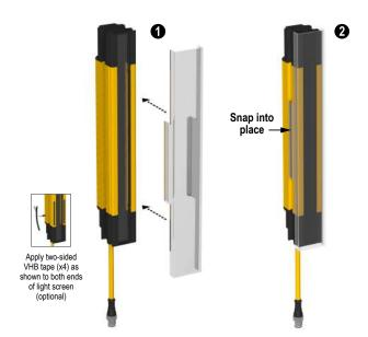
To slide the shield onto the housing:
