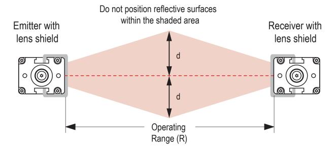
For distance d, with lens shields:
