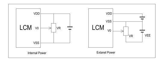
$V_{\text{DD}^{\sim}}V_{0}\text{: LCD}$  Driving voltage
