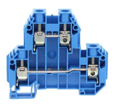
Double-level terminal, Screw connection, Mounting type: Mounting rail TS 35/7.5, Rated cross-section: 10 mm², Width: 10.1 mm, Colour: Blue
