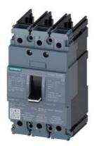
molded case switch 3VA5 UL frame 125 max short-circuit curr. rating 65kA a 480 V 3-pole MCS110, In=100A without overload protection SELF PROTECTION Ii=16 x In Al-lug, line side
