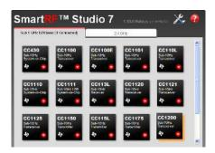
After installing the tool, connect the EB to the PC using the USB cable and start SmartRF Studio. Select the "Sub 1 GHz" tab and double click the highlighted CC1200 device icon.
