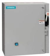
2-speed 3-phase motor starter Size 0 Two separate windings Constant or variable torque Solid-state overload relays Low SPD OLR range 0.75-3.4A High SPD OLR range 3-12A 110V 50HZ / 120V 60HZ coil Combination type 30Amp disconnect switch Enclosure NEMA type 4/12 Water/dust tight for outdoors
