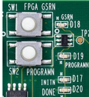
Figure 3. LatticeECP3 Status LEDs and Push-button Controls
