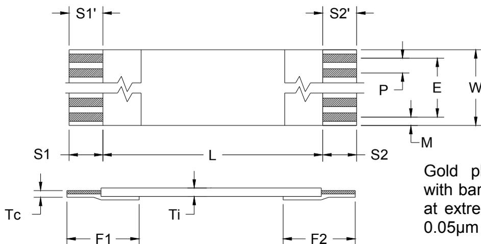
Gold plated conductor is made with bare copper with flash of gold at extremities:  $0.3 \mu\text{m Ni min}$  and  $0.05 \mu\text{m AU min}$ .
