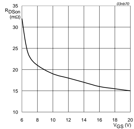
Fig 6. Drain-source on-state resistance as a function of gate-source voltage; typical values.
