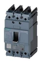
circuit breaker 3VA5 UL frame 125 breaking capacity class M 35kA @ 480 V 3-pole, line protection TM230, FTAM, In=70A overload protection Ir=70A fixed short-circuit protection Ii=5...10 x In UL 489 SB (naval), 50° C without connection
