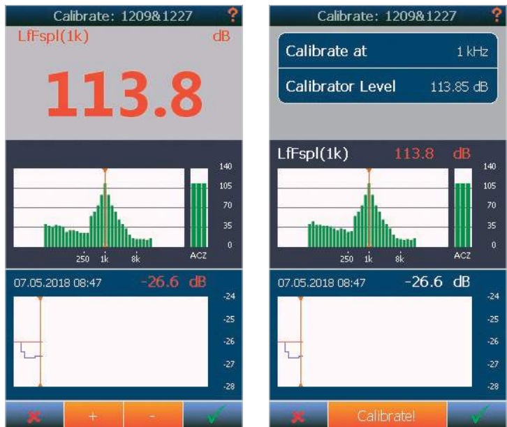
The Calibration menu - Manual and automatic mode
