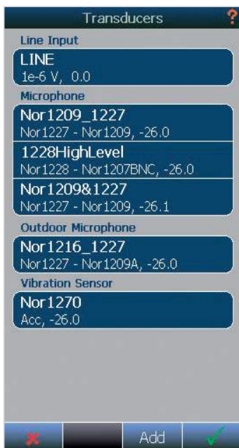
The Transducers menu The calibration history gives you full traceability of the microphone sensitivity.
