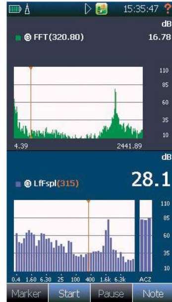
Split view with FFT and 1/3 octave. The link cursor feature connects the cursor in FFT and 1/3 octave displays, making it easy to manoeuvre in the frequency domain
