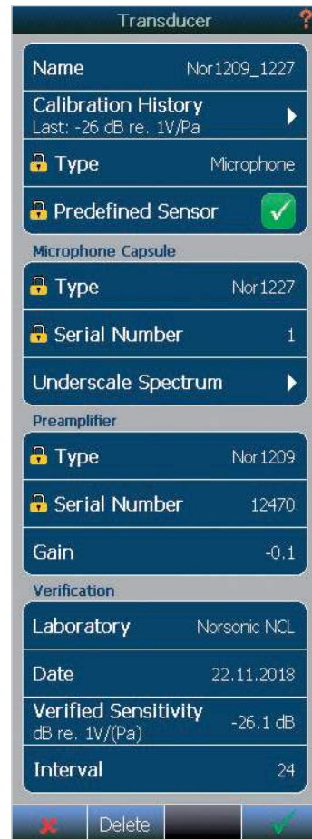
The Transducers menu The calibration history gives you full traceability of the microphone sensitivity.
