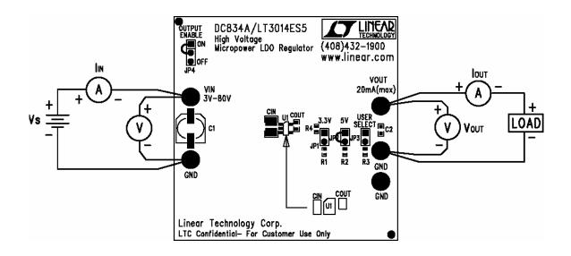
Figure 1. Proper Measurement Equipment Setup
