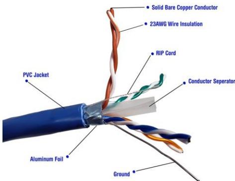
Micro Connectors' Bulk CAT6 Shielded Cable comes conveniently packaged in a pull box, providing you with 1000 feet of high quality, shielded, 4-pair, solid, 550 MHz Cat6 Cable, ready for termination and routing.
