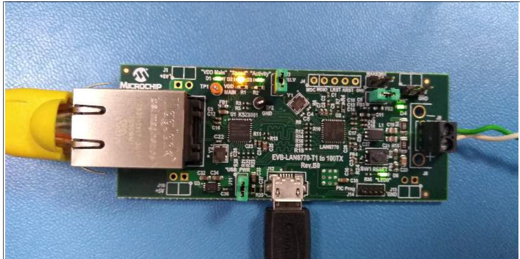
FIGURE 2-1: EVB-LAN8770M_MC EVALUATION BOARD CONNECTIONS
