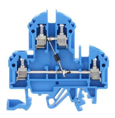
Double-level terminal with electronic components, Screw connection, Mounting type:Mounting rail TS 35/7.5 and TS 32, Rated cross-section: 4 mm², Width: 6 mm, Colour: Blue
