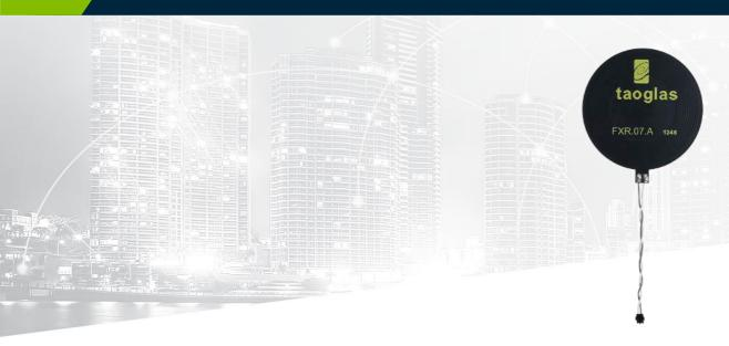
The FXR.07.52.0075X.A is a circular, flexible, NFC (Near Field Communications) antenna for use in mobile devices and other applications such as keycards, payment systems, and boarding passes. The design provides a flexible NFC antenna with 75mm twisted pair 28AWG cable that can be adhered to the plastic enclosure of the device for ease of installation and work with specific 13.56MHz RFID and NFC chips which need to connect via JST ACH connector.
