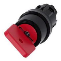
Key-operated switch O.M.R, 22 mm, round, plastic, lock number 73037, red, with 2 keys, 2 switch positions O-I, latching, actuating angle 90°, 10:30h/13:30h, key removal O+I, with laser labeling, upper case and lower case, always upper case at the beginning of the word
