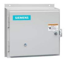
Non-reversing motor starter, Size 1, Three phase full voltage, Solid-state overload relay, OLRelay amp range 0.75-3.4a, 550/575 600 50/60HZ coil, Non-combination type, Enclosure type 12, Dust/drip proof for indoors, Standard width enclosure
