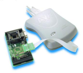
The JTAG ICE interface is integrated in AVR Studio, Atmel's front-end tool for development on the AVR architecture. All phases of the AVR development can be done in this Integrated Development Environment.
