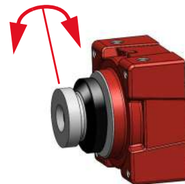
Figure 8: Checking lens is safely locked
