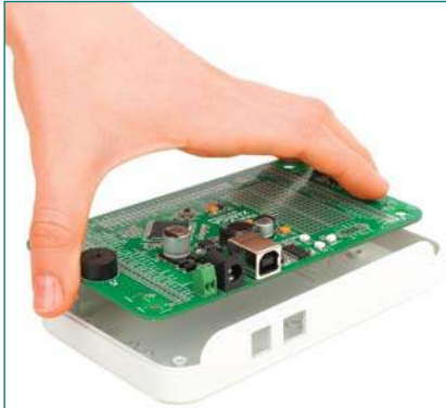
Figure 9-1: Place the board into the bottom part of the casing. Make sure to align the connectors with the square openings
