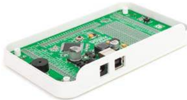
Figure 9-2: Wind screws into inner screw holes to mount the board to the bottom casing plastic
