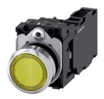
Illuminated pushbutton, 22 mm, round, metal, shiny, yellow, pushbutton, flat, momentary contact type, with holder, 1 NO+1 NC, LED module with integrated LED 110 V AC, screw terminal
