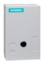
Non-reversing contactor, Size 1 3/4, Three phase full voltage, Contactor amp rating 40A, 3 wire (NO aux included), 190-220/220-240V 50/60Hz coil, Non-combination type, Enclosure NEMA type 1, Indoor general purpose use, Standard width enclosure
