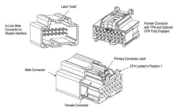
Optional CPA is locked in Position 1 for shipping and handling before engaging the primary connector latch. CPA can NOT move forward or backward until the connectors are mated and the primary latch "clicks" and engages the interface latch tooth.
