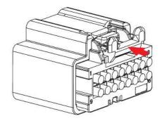
Finally, push the CPA forward to engage secondary lock and ensure proper CPA locking.
