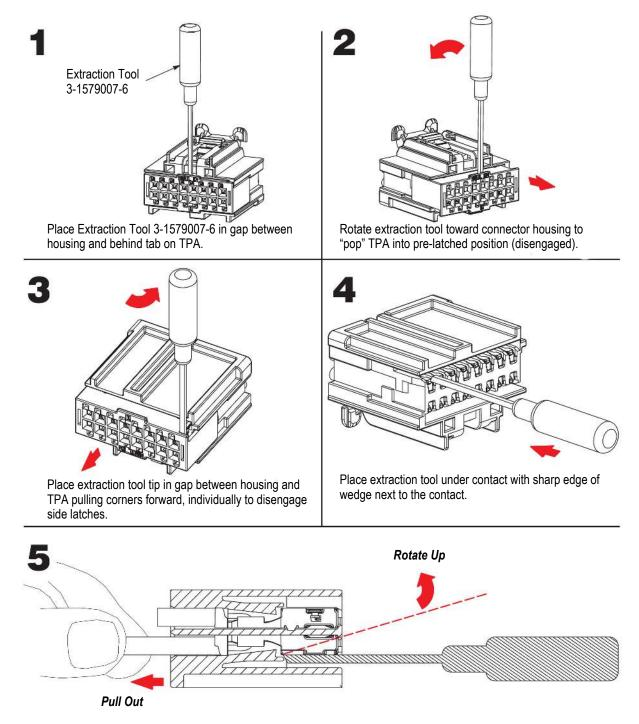
Gently press tool toward the contact latching beam while simultaneously pulling on the wire.
