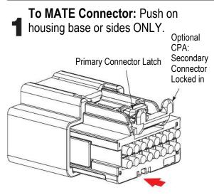
Do not push CPA forward until primary connector latch "clicks" and engages the interface latch tooth. Repeat. 2 To LOCK CPA After Connector Mate : Push CPA forward until an audible "click" is heard.
