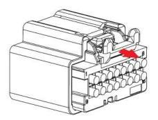
**2 To UNMATE Connector:** With CPA in Position 1, DEPRESS Primary Connector Latch, then simultaneously pull connector/wires while gripping the housing with thumb, index finger, and palm (wire bundle).
