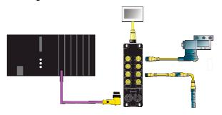
Contained in a 60mm wide housing rated for IP67 environments, BradControl I/O modules can be machine mounted and are able to withstand areas where liquids, dust or vibration may be present. This makes them ideally suited for many applications including material handling equipment and automated assembly machinery.
