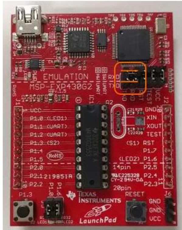
Figure 3. MSP-EXP430G2 Jumper Settings
