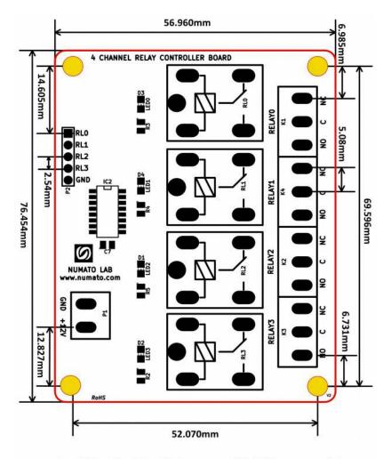
L x W x H : 76.454 mm x 56.960 mm x 20 mm Mechanical Hole Diameter : 4.0 mm
