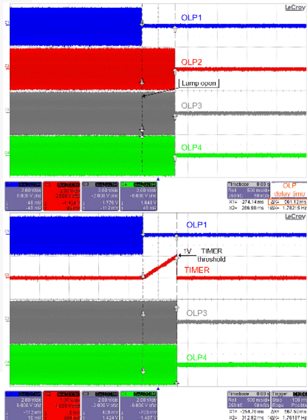
Figure 54. Open-Lamp Protection in Normal Mode
