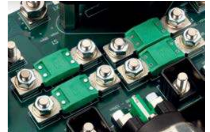
Attaching a megafuse on two M8 male thread PowerElements
